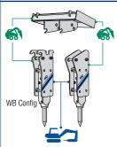
Breakers shown "WB" & "ME" with 2-position pin on Quick-Attach Bracket
