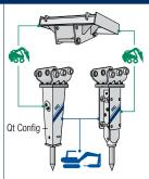
Breaker shown as "Qt" & "FSP" with 2-position pin on Quick-Attach Bracket
